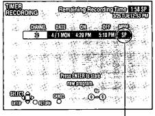
The current recording mode (shown on the unit's display) is automatically selected. In case where the recording mode has already been set to XP, the recording mode will be automatically changed to FR mode.
